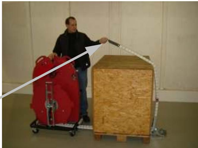
.... move the Chain Lance completely backwards by pushing the joystick in the “move in“ direction.
