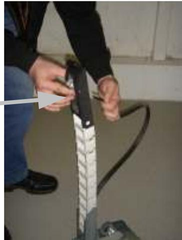
Push the strap from the back through the top of the ChainLance as shown. The packaging strap must be pushed under the eccentric latch.
