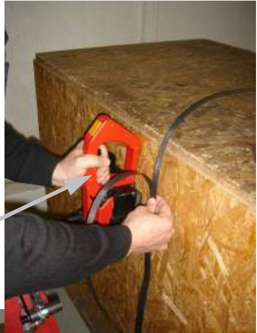
With your right hand you can now feed the strap from the top to the bottom through the slot in the sealing tool.
