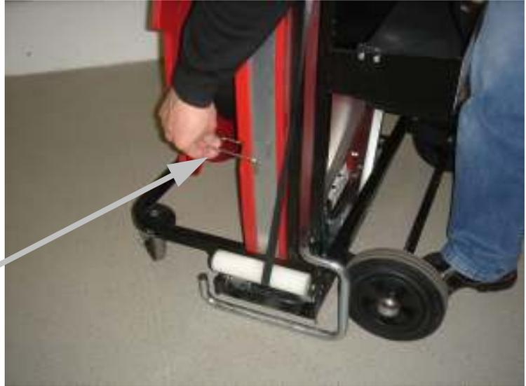
...and set the package width as shown. Plug the clamp into the next highest dimension of your package width.
