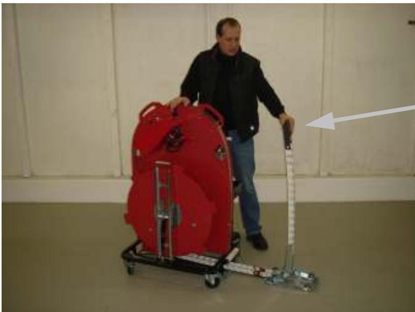
Hold the end of the ChainLance with the left hand while you still continue to push the joystick in the “move out direction“.
