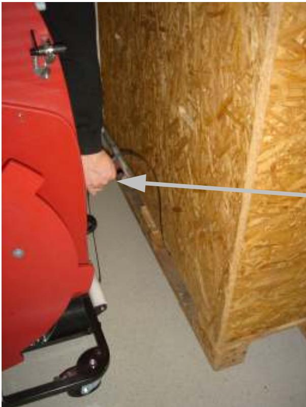
...but about 10 cm below the strap lifter. Hold the strap with the whole hand and pull it out of the unit. You also have to let the end of the strap slide through your other hand at the same time!
